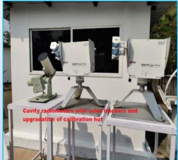
Fig. 8. Cavity radiometers with solar trackers and upgradation of calibration
