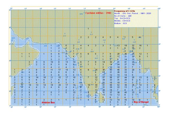
Fig. 4.4. Frequency of all Cyclonic disturbances (Depressions and above) during the period 1961-2020. In each box top figure shows the frequency of Dep+CS+SCS, middle one CS+SCS and bottom one is the frequency of SCS. These statistics is derived from IMD Cyclone atlas.
