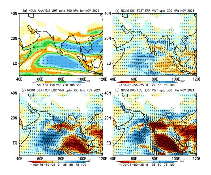
Fig. 8.2. a) The NCUM model analysis of vertically integrated (up to 300 hPa) moisture transport (VMT) during Nov 2021. The forecast error in VMT for day-1 (b), day-2(c) and day-3(d).
