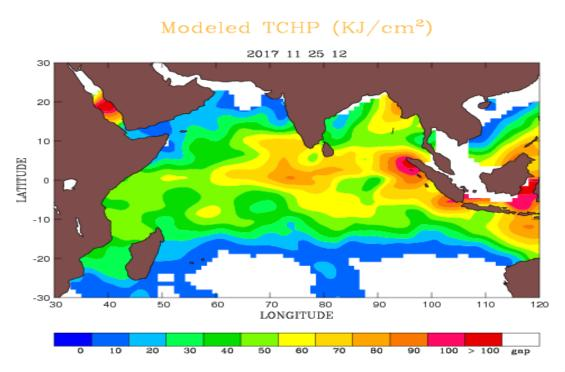
Fig. 4.19. Spatial distribution of Tropical Cyclone Heat Potential (TCHP) in KJ/Cm<sup>2</sup> on 25 November 2017, just prior to the formation of TC-OCKHI. Source: NRSC, ISRO.
