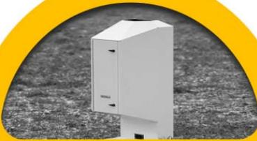
**1974:** Ceilometer was installed to estimate the height of the base of the low clouds at Mumbai.
