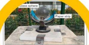
**1962:** A Sunshine recorder is a device that records the amount of sunshine at a given location at any time.
