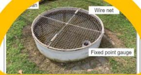
**1962:** This pan evaporimeter also known as modified Class A Pan, consists of a pan 1207 mm in diameter with 250 mm of depth.
