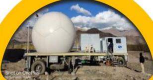
**2021:** A transportable X-band Doppler Weather Radar mounted on a mobile platform was installed at Leh. The Leh DWR installed by IMD is at the highest altitude in India.
