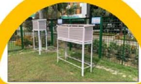
**1962:** Stevenson screen is a shelter to meteorological instrument and allows air to circulate freely around them.
