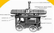
**1928:** First Observations of Total Column Ozone in India at Kodaikanal using Dobson Spectrophotometer with the permission of the DGO in India
