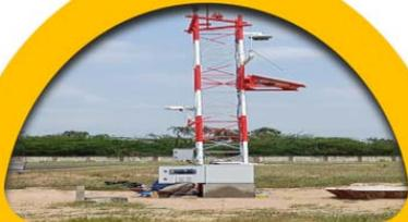
**2022:** Helicopter Aviation Weather Observing Systems (H-AWOS) installed by IMD over a heliport.
