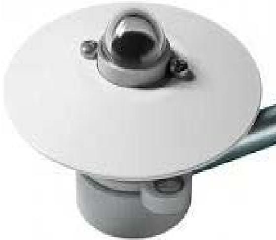
The sensor uses a thermocouple junction. A copper constantan Thermo junction is created on top and bottom surface. The Top surface is coated with optically black paint for absorbing 98% of solar Radiation with reference to black body. The Top surface absorbs solar Radiation and acts as a hot junction. The bottom surface in shadow acts as a cold junction. A hemispherical glass dome on the sensor allow only short wave Radiation coming from Sun.
