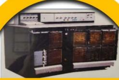
**1973:** IBM 360/44 used for processing MONEX data. It had memory of 512KB with CPU speed-4MHz along with storage capacity of 64MB.
