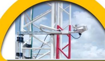
**2021:** Forward scatterometer type RVR system installed at New Delhi airport.
