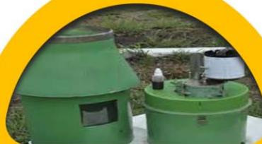
**1970:** Self-recording raingages (SRRG) record the rainfall depth in the form of a continuous plot.
