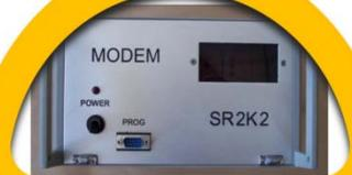
**2002:** System Reception (SR2K2) is a ground instrument for reception of data from sonde.
