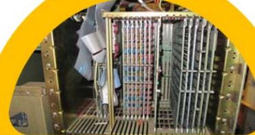
**1988:** A family of 32-bit superminicomputers, running the Virtual Address eXtension (VAX) instruction set architecture (ISA) is used for communication.
