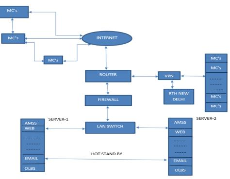
Figure 2. Data Flow of AMSS
