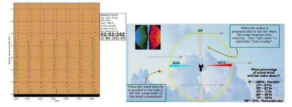
VVP-2 product of DWR. The concept of DWR radial wind & "Zero Isodop"
