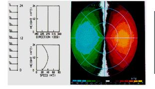
In the second example, the winds increase from 20 to 40 knots between zero and 12,000 feet and then decrease again to 20 knots at 24,000 feet. The <u>wind</u> <u>direction</u> again is constant. The radar beam intersects the 12,000 foot level along a ring half-way across the radar display. This is where we see the maximum inbound and outbound velocities.
