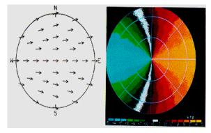
In the third example, we see a wind field which changes direction from north to south but has a constant speed at all heights. The zero radial velocity line now bends so that it is everywhere perpendicular to the wind field. The maximum <u>radial velocities</u> are observed where the radar beam points directly toward or way from the wind direction.
