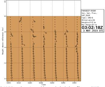
Fig. 7. VVP2 product. It provides vertical wind profile over DWR station
