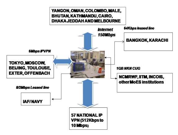
Figure 6. Telecommunication Infrastructure of IMD
