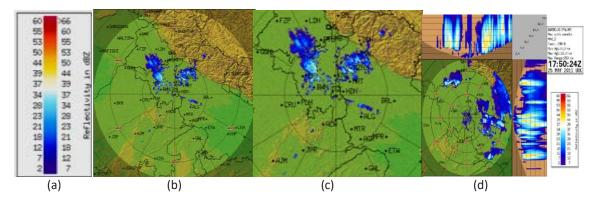
Figure. (a) The IMD DWR Reflectivity colour coded Scale (b) Reflectivity PPI-Z image (c) The close range reflectivity PPI-Z image and (d) Reflectivity MAX-Z Image
