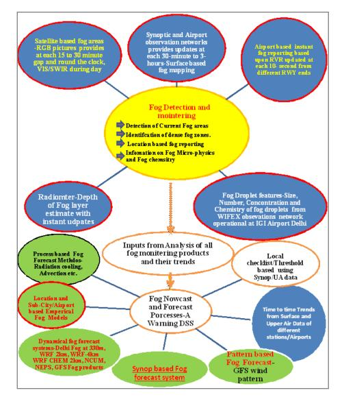
Figure 8b. Block diagram of present Fog Monitoring, Nowcasting, and Forecasting System functional in IMD 187
