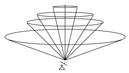
Fig. 2. Radar Volume scan
