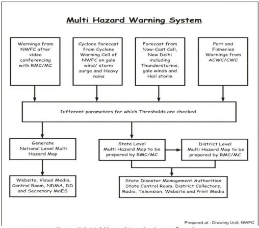
Figure 10.2. Multi hazard Warning System flow chart
