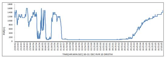
Figure 5. Integrated Rwy Vis display system of IGIA where Fog status is reported at each instant of time and updated at each 10 second(Top one). Instument Vis values–RVR for a dense fog date at IGIA
