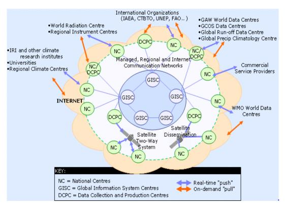
Figure 4. Diagram showing WIS core components and Information Exchange
