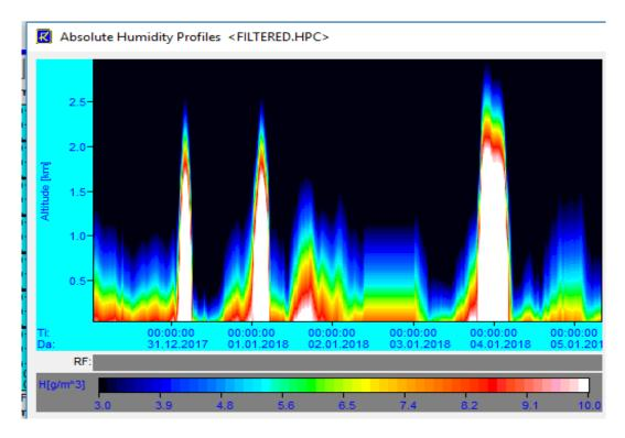
Figure 7. Micro- wave Radiometer captures fog layer in terms of moisture profiling at each instant. It captures the dense fog spell prevailed over IGI Airport Delhi during 30 De-5 Jan 2017-18 with day to day variation of time of onset, depth of fog layer and lifting
