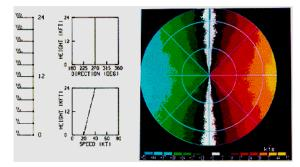
For this first example, wind is constant with height, but <u>wind speed</u> increases from 20 knots at the ground to 40 knots at 24,000 feet. Note on the velocity field the maximum inbound velocity is to the west and maximum outbound is to the east while to the north and south the radar measures zero radial velocity. This is because the winds are perpendicular to the radar beam when viewed to the northor south.
