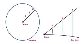
On a radar PPI display, the distance away from the radar at the center of the display represents both a change in horizontal distance and a change in vertical distance. To determine the wind field at a particular elevation above the radar, one must examine the radial velocities on a ring at a fixed distance from the radar. The exact elevation represented by a particular ring depends upon the elevation angle of the radar beam.
