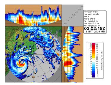
Fig. MAX-Z product from Doppler Weather Radar. Provides location as well as height of clouds
